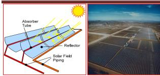
Fig.2 Solar Collector
